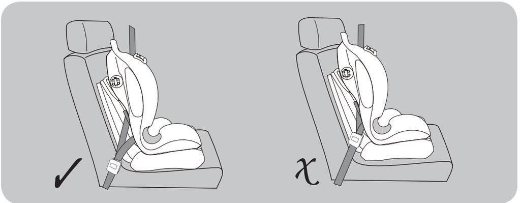
With your child car seat now buckled in, check it is secure by pulling forward from both harness straps, there should be little or no movement. Next check that the vehicle's seatbelt buckle is **NOT** resting against the child car seat shell. This is called 'buckle crunch' and could cause the child car seat to work loose or the seatbelt to come undone in an accident. If you find you are experiencing 'buckle crunch' then this child car seat is not suitable for your vehicle.
