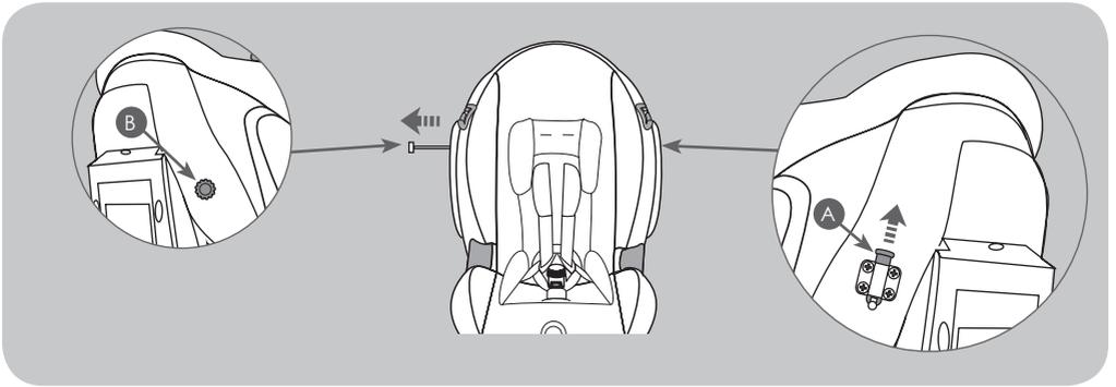
Pull up lock (A) on the top right hand side of the shell and pull out the installation bar (B) on the opposite side.
