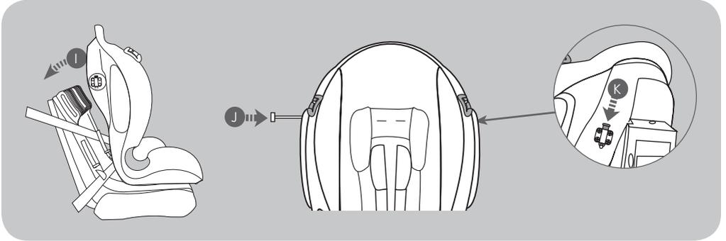
Return the shell to its original position (I) taking care not to trap the diagonal shoulder belt and thread the installation bar back through the seat (J). Secure the lock on the top right hand side of the child car seat (K). Pull the installation bar to ensure it is securely locked in place.
