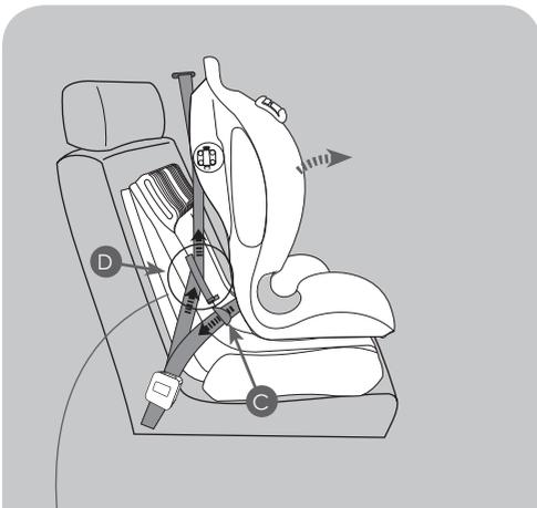
Tilt the seat shell forwards, feed the seatbelt between the seat and the base and plug the buckle in ensuring the seatbelt is not twisted.
