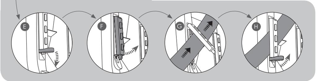
To operate the lock-off device: Pull down on tab (E) to open the locking device. Lift up the latch (F). Pass the seatbelt under the latch and pull the belt tight (G). Close the latch and fasten the tab (H) whilst holding the diagonal section of seatbelt tight.
