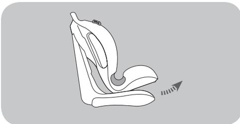
Place the child car seat on a suitable passenger seat. Adjust the child car seat to its most reclined position.
