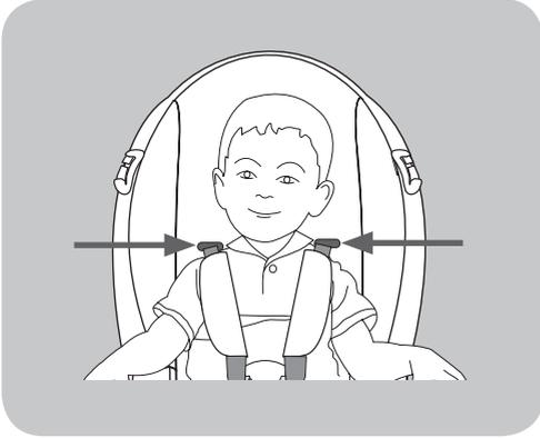
The harness strap slots should be level with or above your child's shoulders. If they are not, then you may need to reposition the harness shoulder straps and adjust the harness height.
