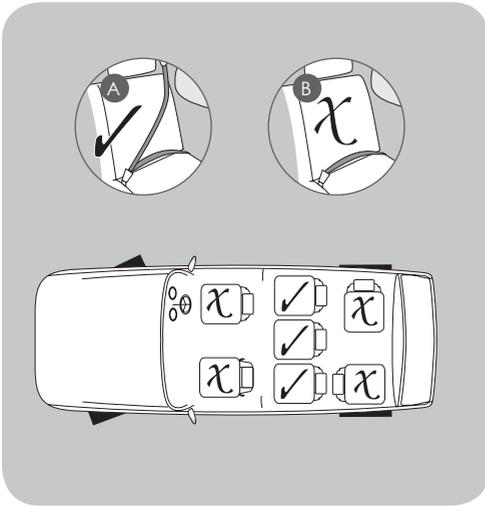
The child car seat can only be used with an automatic 3-point safety belt (A) and **NOT** with a 2-point lap belt (B).
