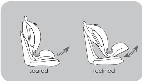
The child car seat can be used in five different seat positions, from seated to a reclined sleeping position. Pull the recline adjuster handle under the front of the shell and whilst holding it, pull the shell forwards or backwards, release the handle on your required position when hearing a distinct click.
